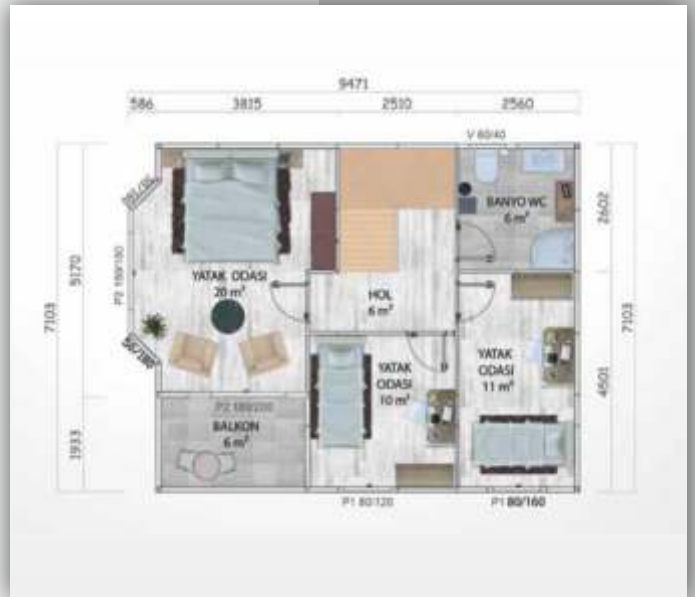
66m 2 (60 m 2 + 6m 2 BALKON) 1. KAT PLANI 66m 2 (60m 2 + 6m 2 Balcony) First Floor Plan
