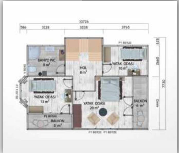
77m 2 (66 m 2 + 11m 2 BALKON) 1. KAT PLANI 77m 2 (66m 2 + 11m 2 Balcony) First Floor Plan
