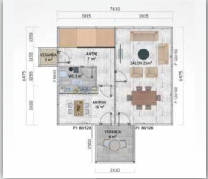
58m 2 (50m 2 + 8m 2 VERANDA) ZEMİN KAT PLANI 58m 2 (50m 2 + 8m 2 Terrace) Ground Floor Plan
