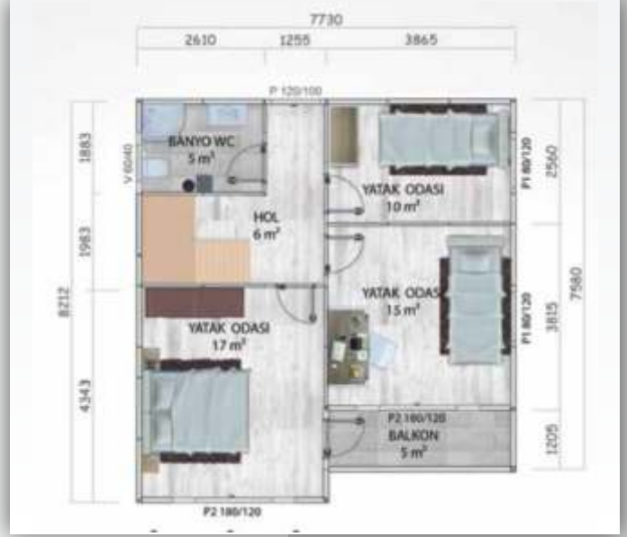
62m 2 (57m 2 + 5m 2 VERANDA) ZEMİN KAT PLANI 62m 2 (57m 2 + 5m 2 Terrace) Ground Floor Plan
