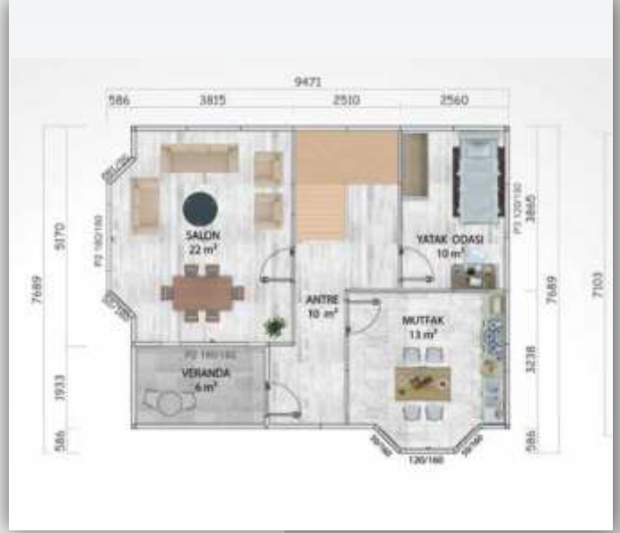
65m 2 (59m 2 + 6m 2 VERANDA) ZEMİN KAT PLANI 65m 2 (59m 2 + 6m 2 Terrace) Ground Floor Plan
