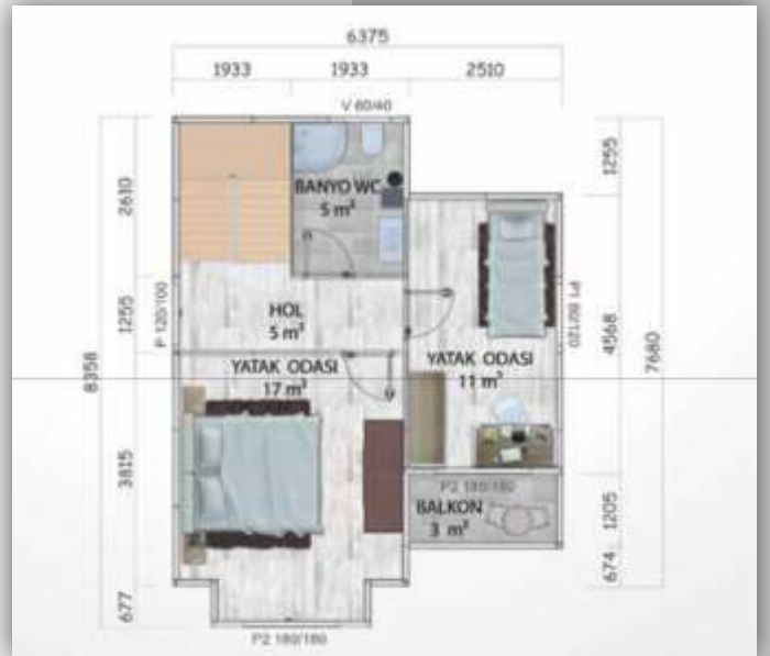
46 m 2 (43m 2 + 3m 2 BALKON) 1. KAT PLANI 46m 2 (43m 2 + 3m 2 Balcony) Frist Floor Plan
