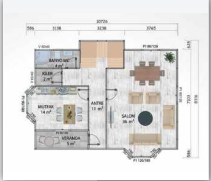
78m 2 (73m 2 + 5m 2 VERANDA) ZEMİN KAT PLANI 78m 2 (73m 2 + 5m 2 Terrace) Ground Floor Plan
