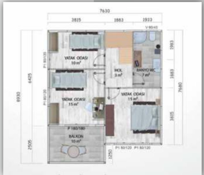
63m 2 (53 m 2 + 10m 2 BALKON) 1. KAT PLANI 63m 2 (53m 2 + 10m 2 Balcony) Frist Floor Plan
