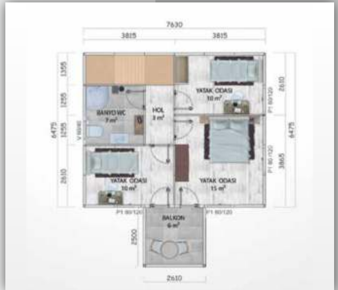
56m 2 (50m 2 + 6m 2 BALKON) 1. KAT PLANI 56m 2 (50m 2 + 6m 2 Balcony) First Floor Plan
